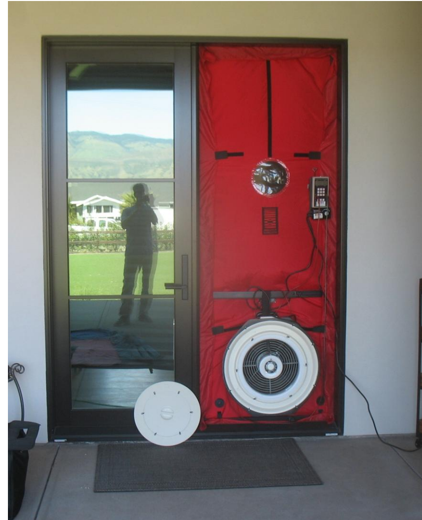
Compartmentalization Testing, i.e. Blower Door Testing
