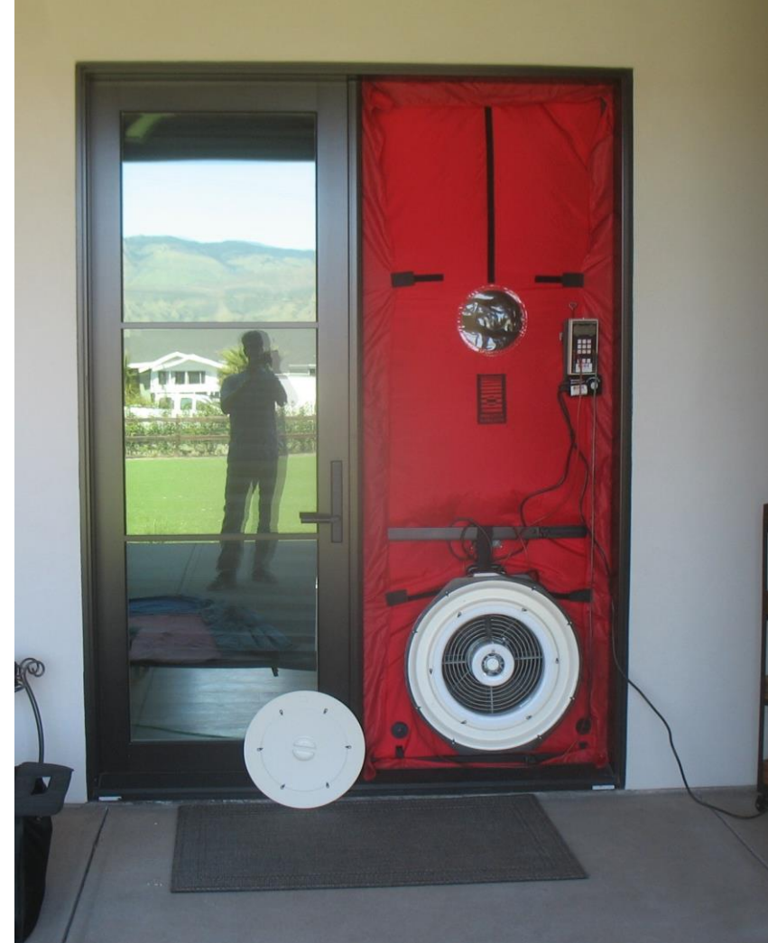
Compartmentalization Testing, i.e. Blower Door Testing
