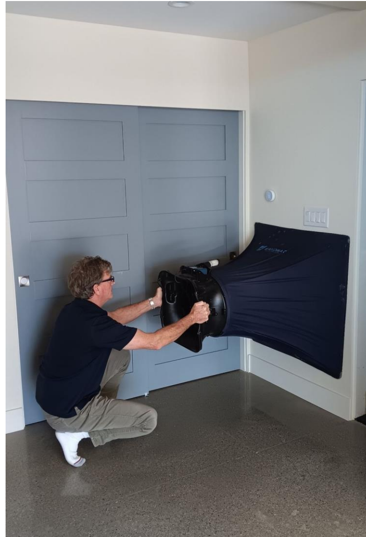
HERS/ECC Rater testing proper air flow with a flow hood.
