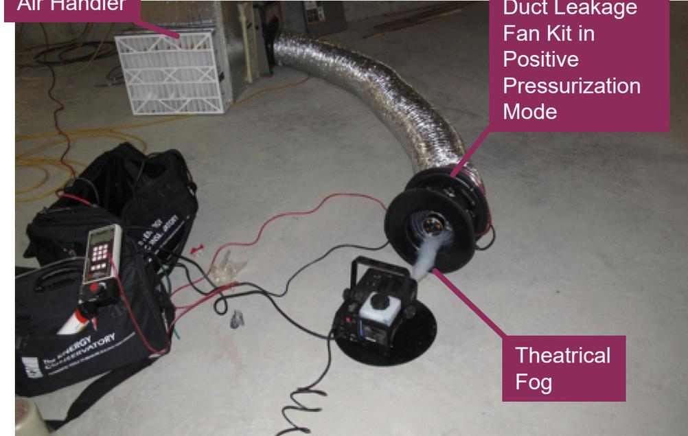
Duct Leakage Fan Kit in Positive Pressurization Mode
