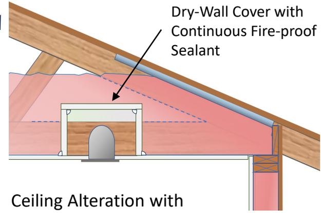
Ceiling Alteration with Existing Recessed Fixture
