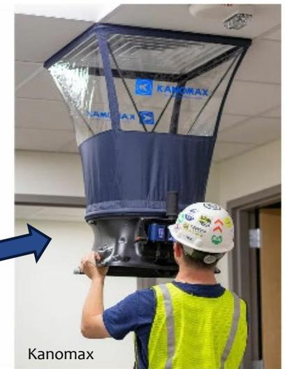
**Flow Capture Hood** Measures the air volume in cubic feet per minute (cfm) at the register.
