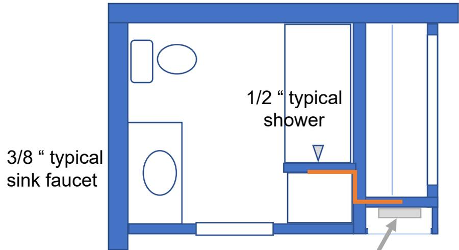
Instantaneous electric water heater with *point of use distribution*
