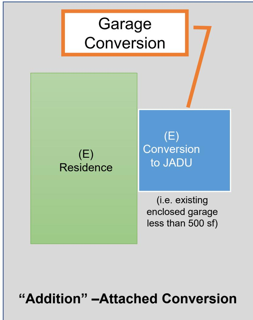
**Junior ADU (JADU) –Conversion of the unconditioned space of an attached garage or attic or basement, etc.**
