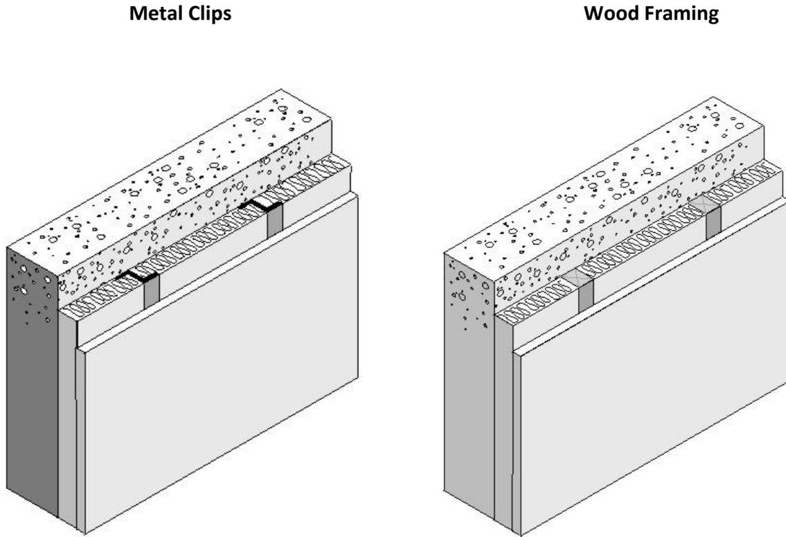
Figure 4.3.14 – Interior or Exterior Insulation Layers
