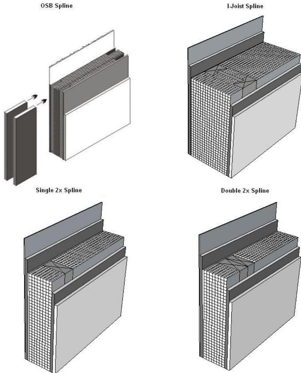
Figure 4.3.2 – Structurally Insulated Wall Panels (SIPS)
