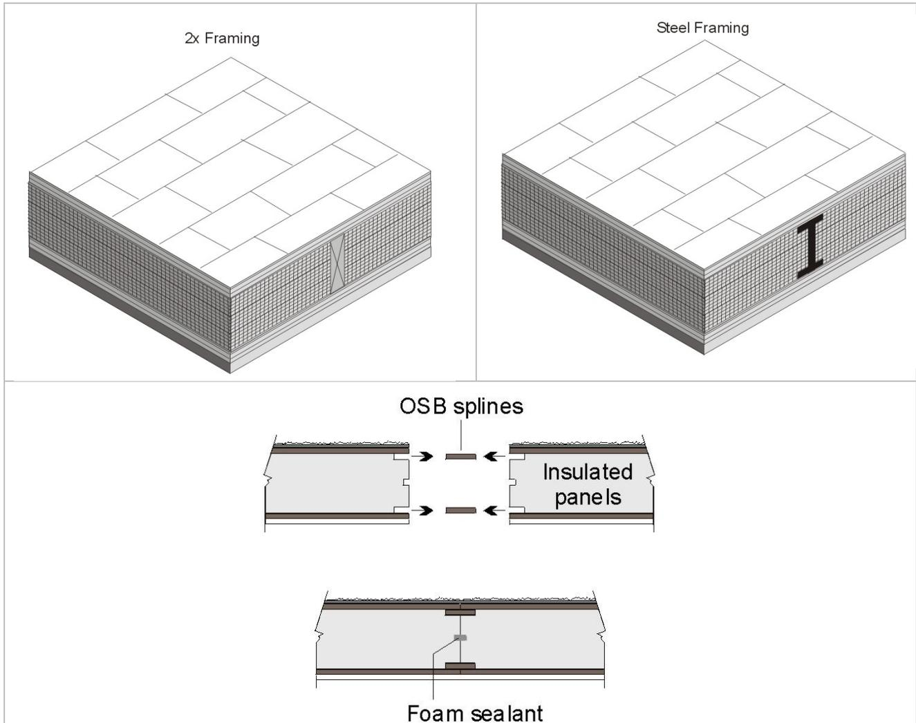
Figure 4.2.3 – SIPS Roof/Ceiling
