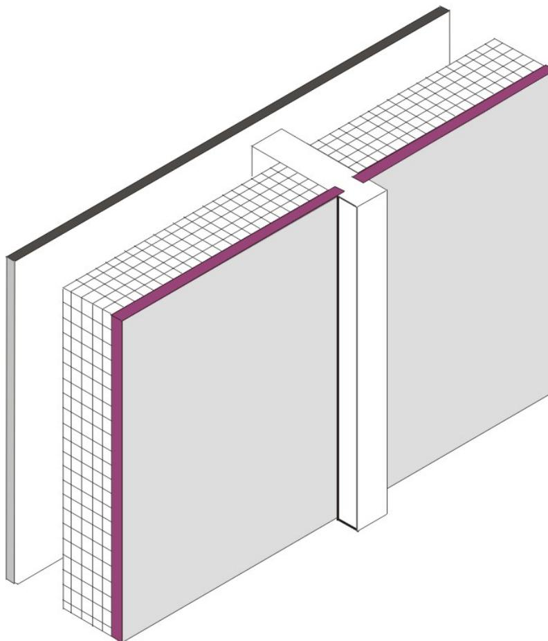
Figure 4.3.8 – Spandrel Panel
