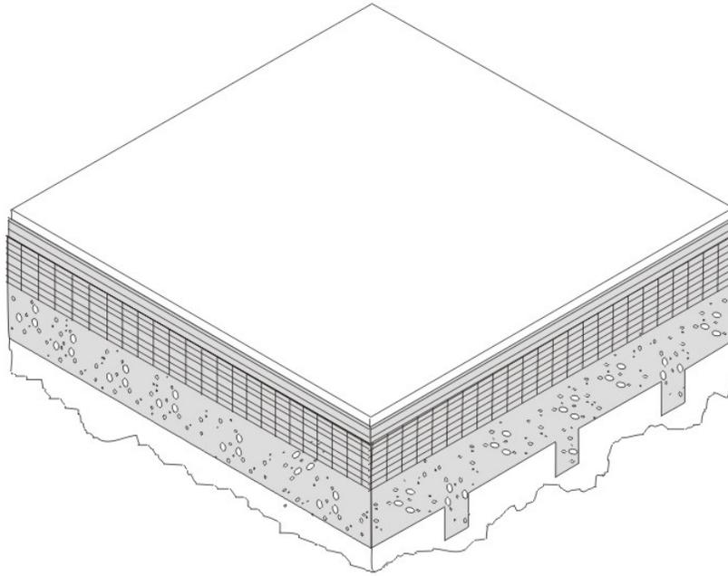
Figure 4.2.6 – Span Deck and Concrete Roof
