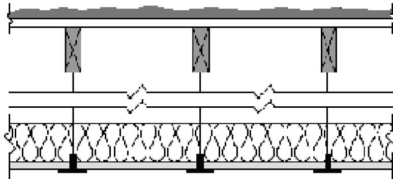
Figure 4.2.8 – Insulated Ceiling with Removable Panels
